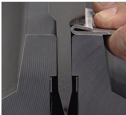
Pre-bend and flattening in the same tool.
